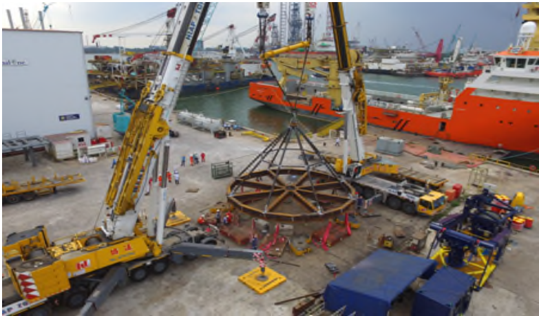
Load Testing for Turret Main Bearing Lifting Frame
