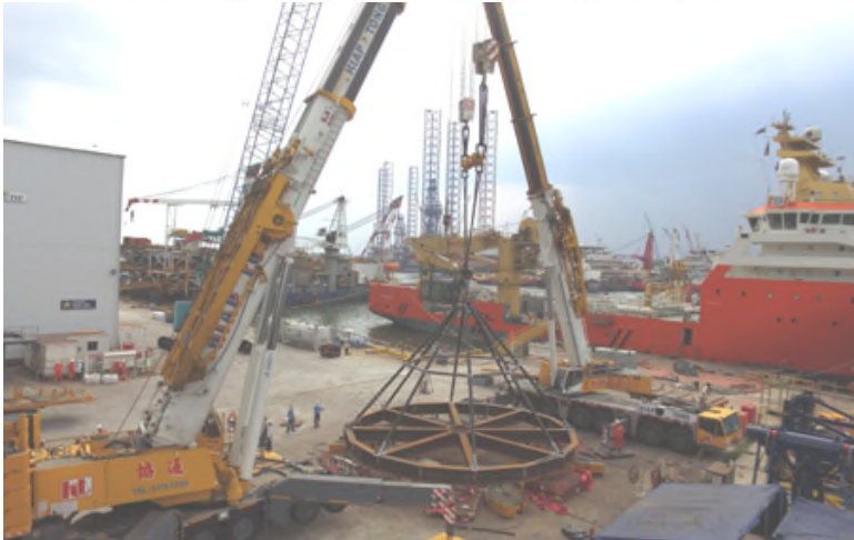
Load Testing for Turret Main Bearing Lifting Frame
