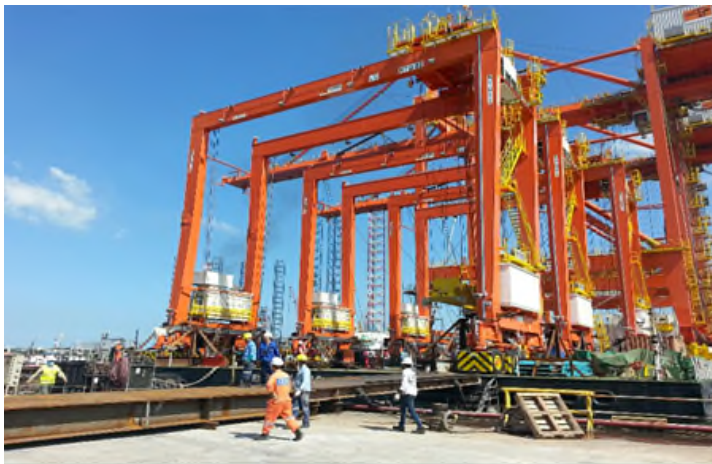
Rubber Tyred Gantry (RTG) Crane Offloading & Repair
