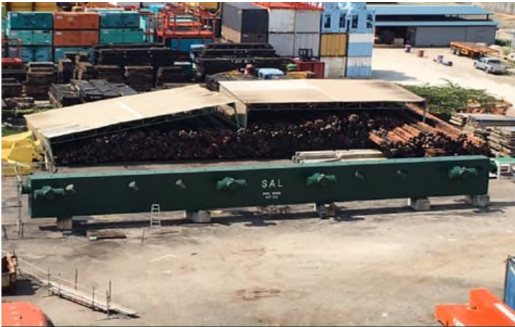
Fabrication & Repair of 1000 Ton Lifting Beam
