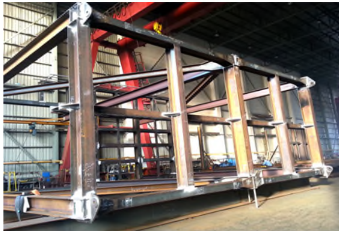
Fabrication of Turret Trolley Support Structure
