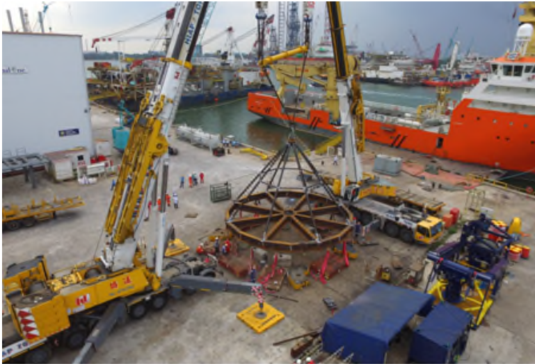
Load Testing for Turret Main Bearing Lifting Frame
